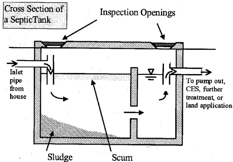
**Figure 2:** Cross Section of a Septic Tank
