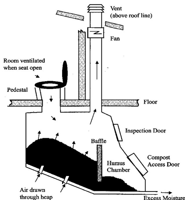
**Figure 7: Cross Section of a Compost Toilet**
