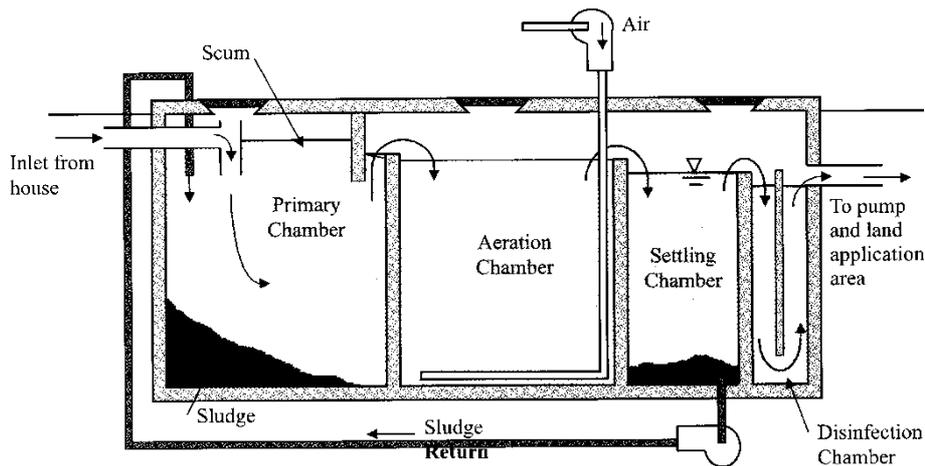
**Figure 3:** Cross Section of an AWTS
