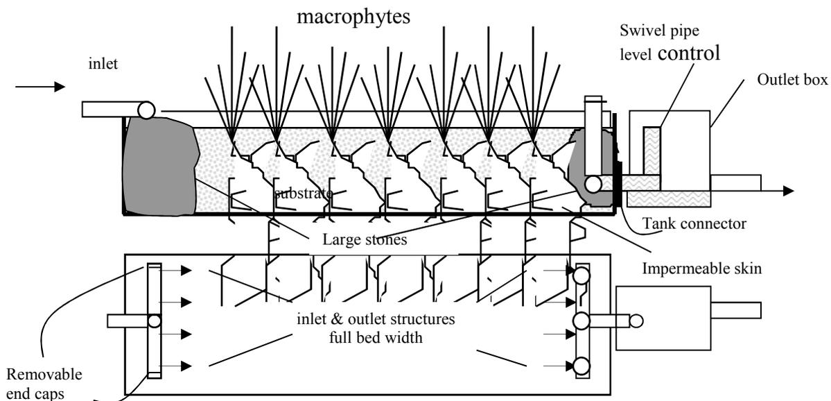
**Figure 6:** Elevation and plan views of typical horizontal subsurface flow wetland showing major components
