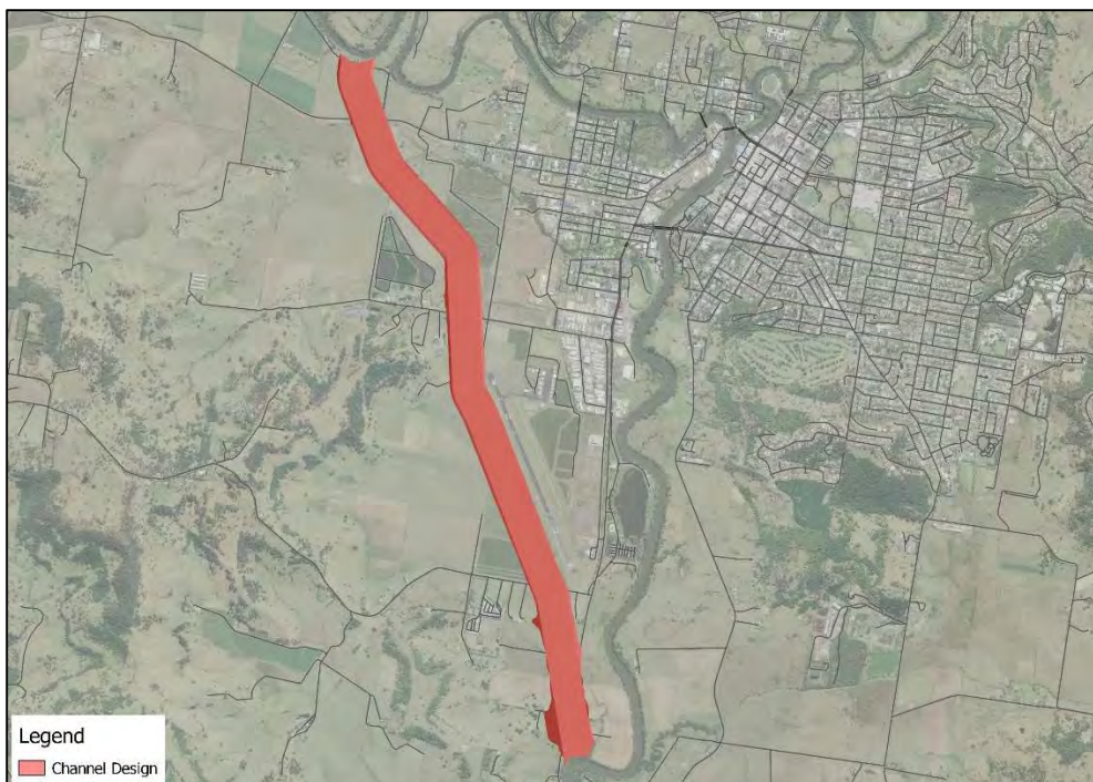
Figure 1 – Leycester Creek Bypass Channel Alignment
