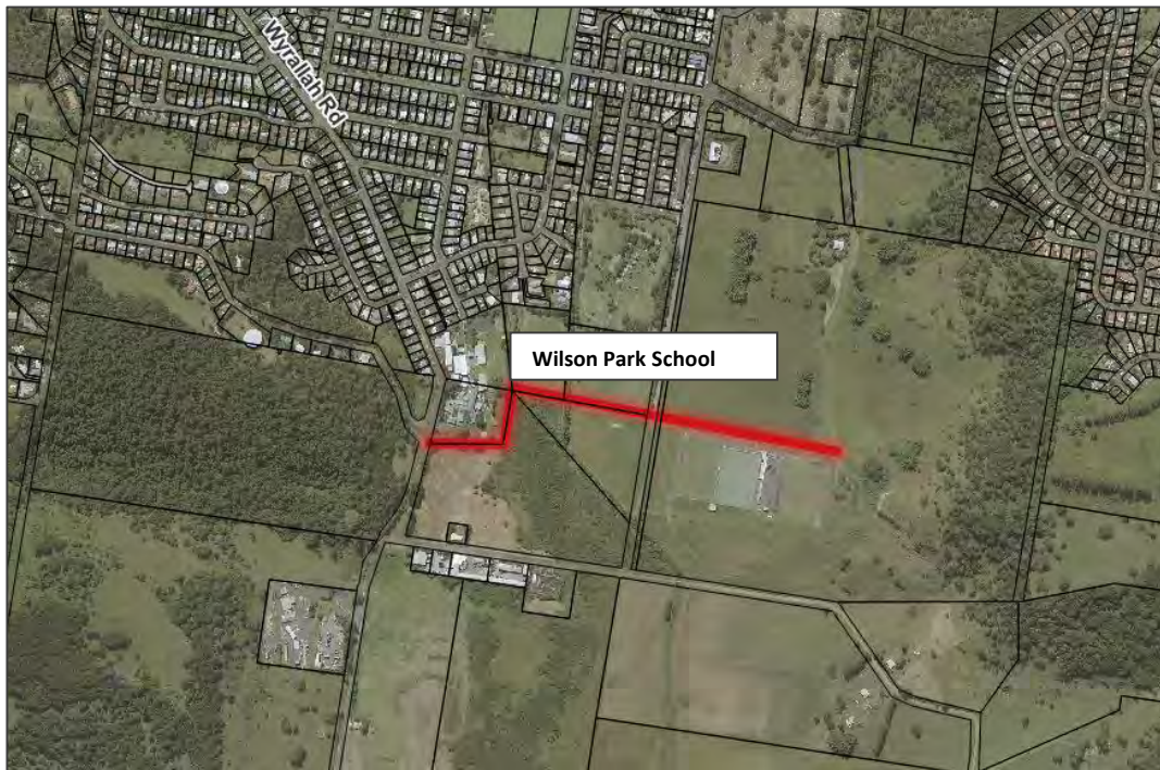
Figure 3: Option 3 Levee Alignment
