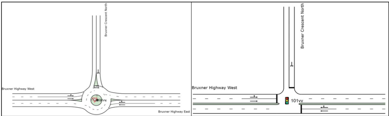
Upgraded SIDRA Model Layouts | Roundabout (left) and Signals (right)
