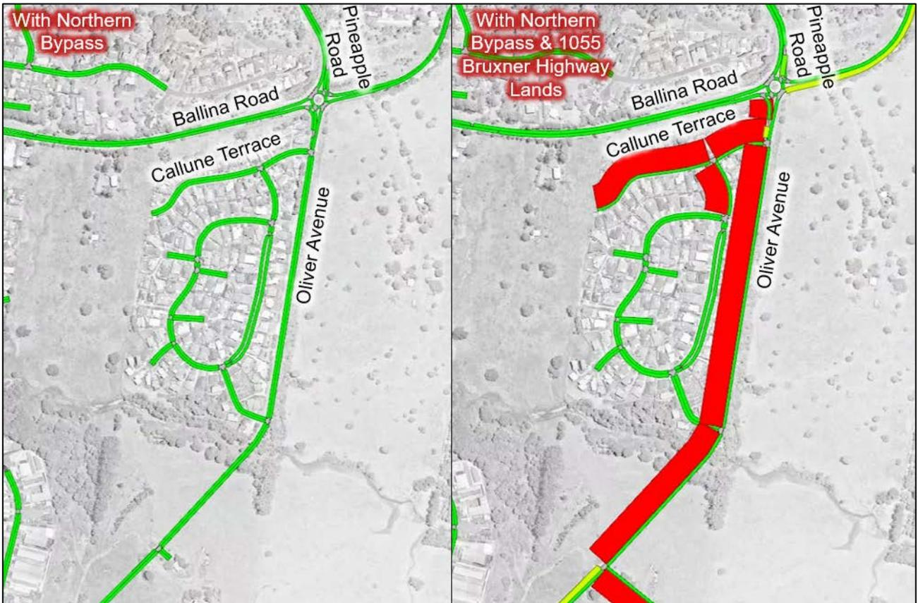
**Figure 4.20: Ballina Rd / Pineapple Rd / Oliver Ave 2038 0800-0900 AM Peak Link Delays**
