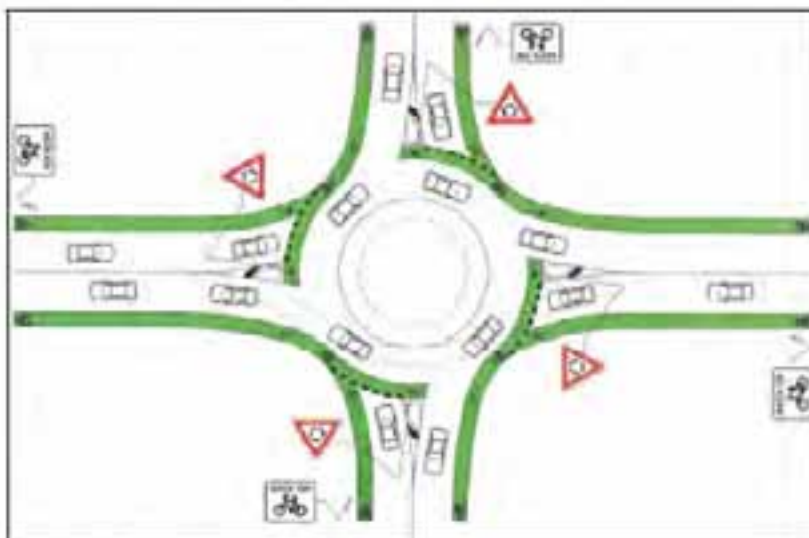
Figure 5.4: Two bicycle routes crossing at a single-lane roundabout with no physical separation of bicycle lanes (some jurisdictions may not favour this treatment – refer Section 5.3.1)
