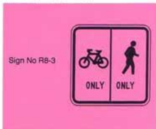
Figure 7.4 Segregated Footway Sign
