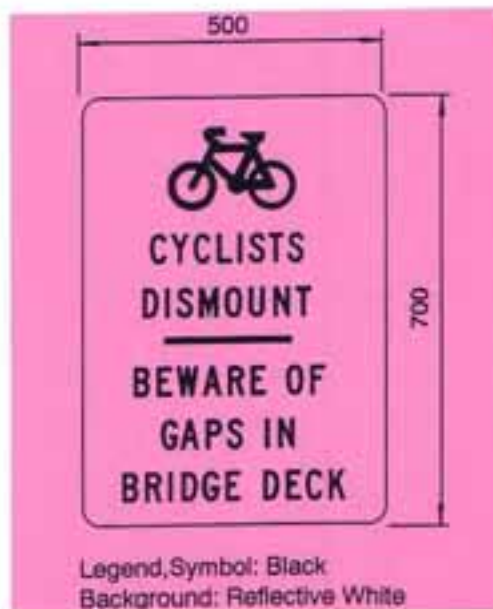
Figure 7.14 Gaps In Deck Sign
