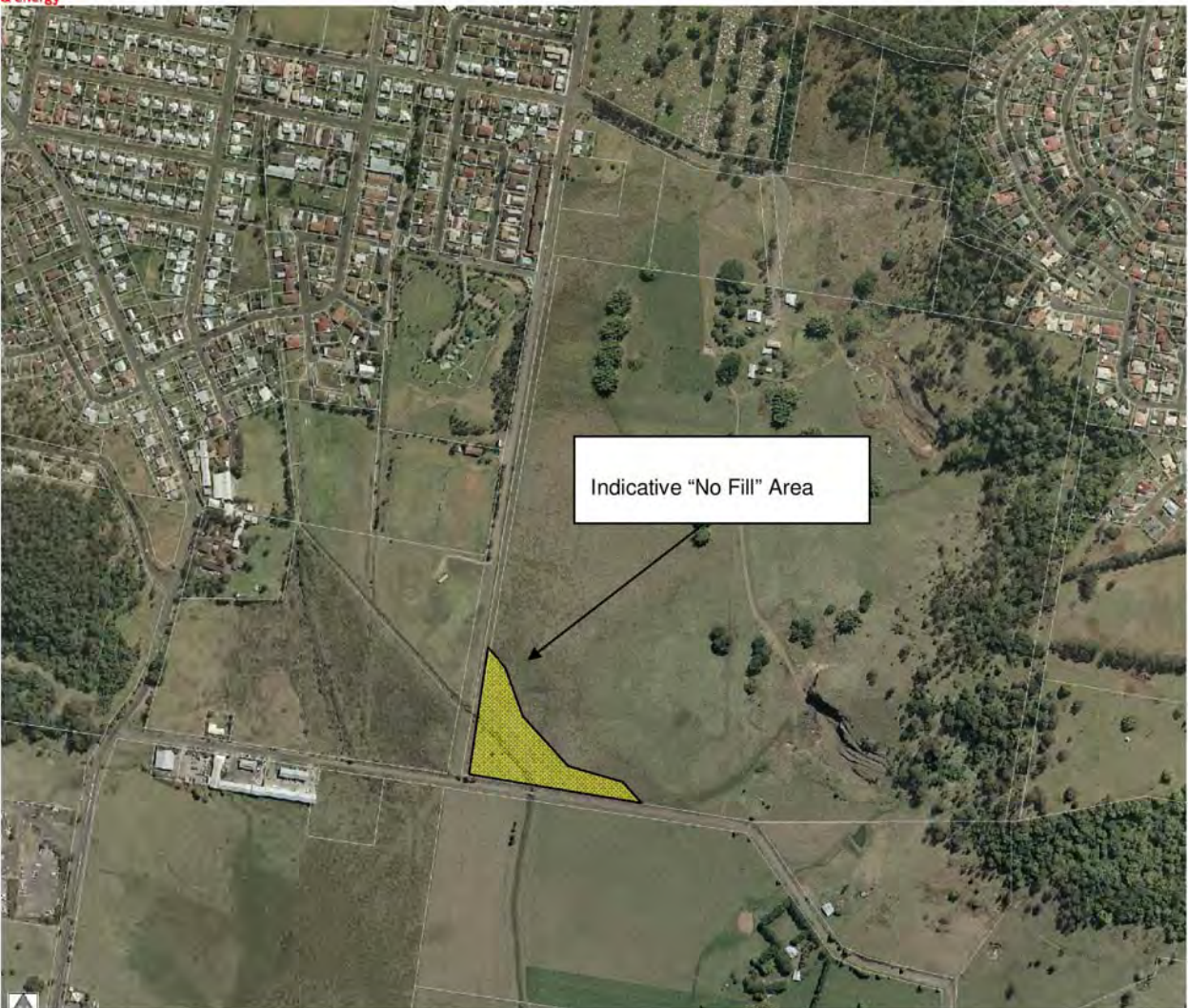
Figure 6 – Indicative “no fill” area to convey Minaltrie Creek local 10yr flows without increasing upstream peak levels.
