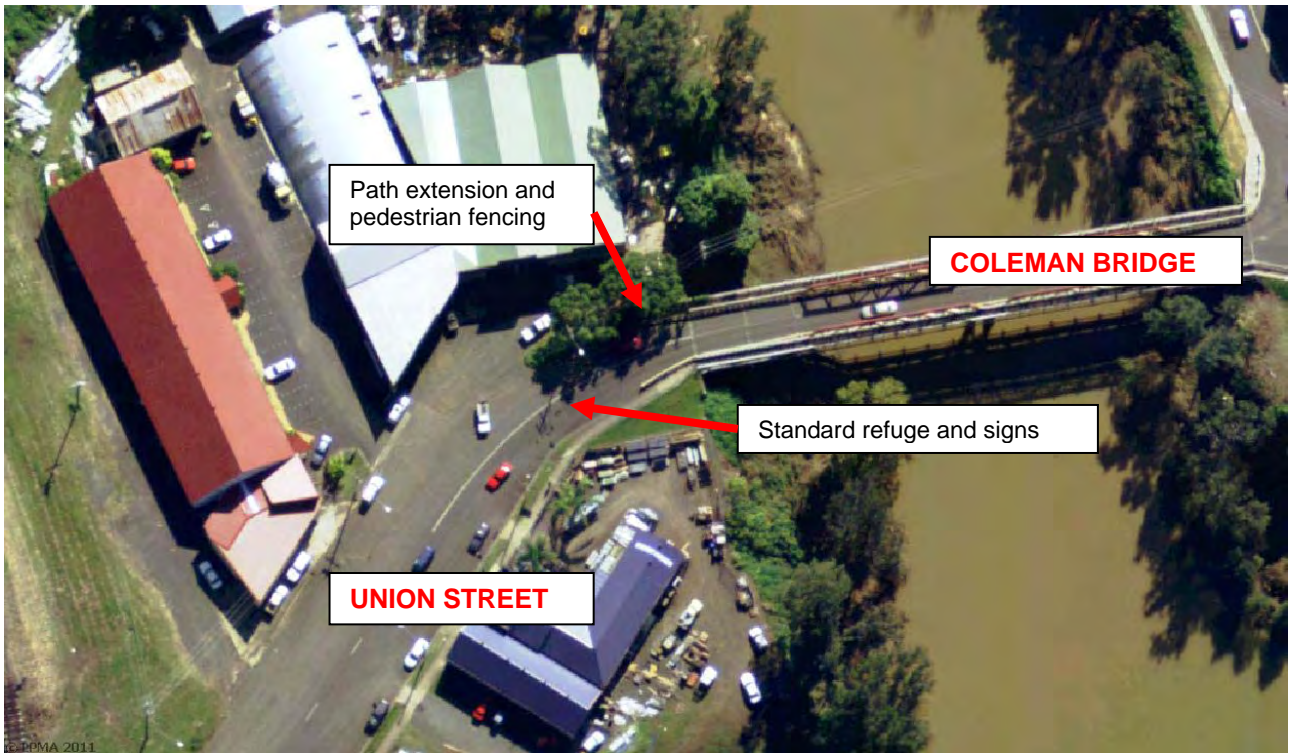
Item 12: Union Street approach to Coleman Bridge
