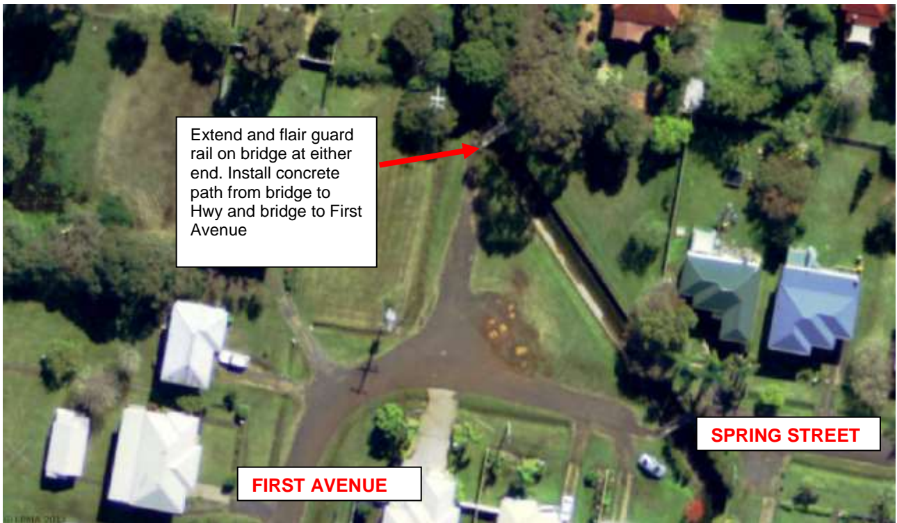
Item 82: First Avenue Pedestrian Bridge
